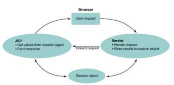
The basic steps for a servlet communicating with a JSP file to present information to a client are as follows:
