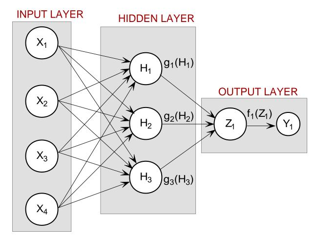
There are a total of 19 weights in this network. The activations functions are all linear. Since the target output is a linear function of the input attributes, linear activation functions guarantee that the network forecasts will exactly match their targets. Of course, this same result could have been obtained using linear multiple regression. Training is conducted using the quasi-newton trainer.
