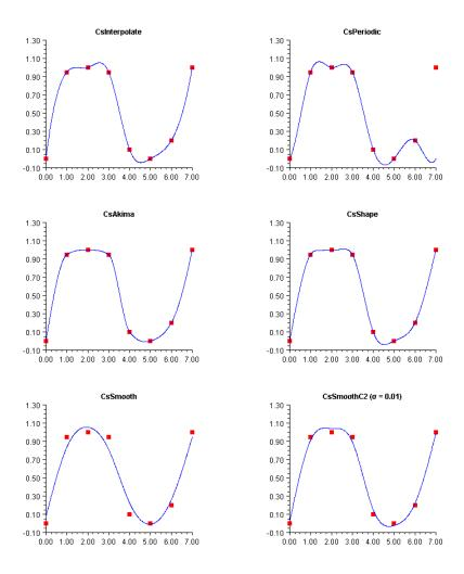
The chart shows how the six cubic splines in this chapter fit a single data set.
