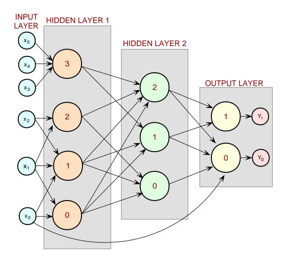
Figure 8. A Three-Layer Feed-Forward Neural Net
