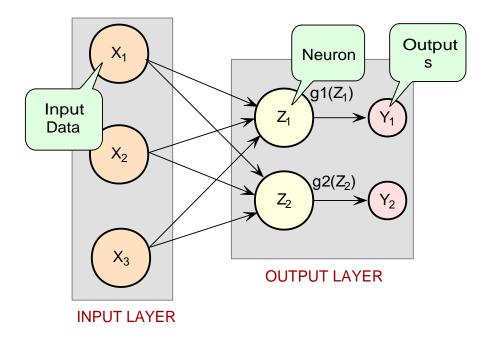
Figure 7. A Single-Layer Feed-Forward Neural Net
