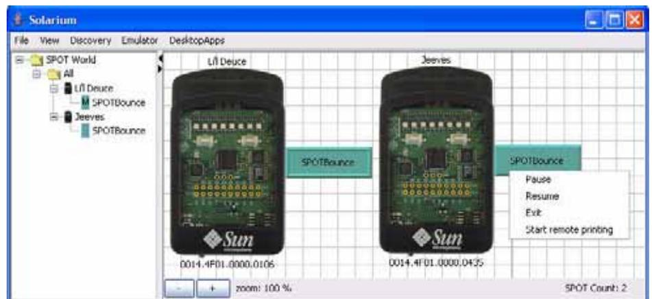
In the illustration, the SPOTs are both running the Bounce demo. The SPOT on the left is running in the main isolate, as shown by **M** in the tree view. The SPOT on the right is running it as a child isolate.
