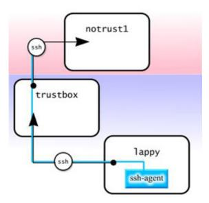
As you can see, when ssh connected to trustbox, it maintained a connection to the ssh-agent running on lappy. When an ssh connection was made from trustbox to notrust1, this new ssh process maintained the authentication connection to the previous ssh, effectively extending the chain. Whether this authentication chain can be extended beyond
