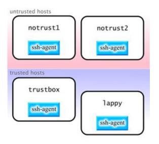
The problem with this approach is that if someone gains root access on notrust1 or notrust2, then it is of course possible for this person to extract keys from the now vulnerable ssh-agent process. To fix this, drobbins stops running ssh-agent and keychain on untrusted hosts notrust1 and notrust2. In fact, to be even more careful, drobbins decides to only use ssh-agent and keychain on lappy. This limits exposure of his decrypted private keys, protecting him against private key theft:
